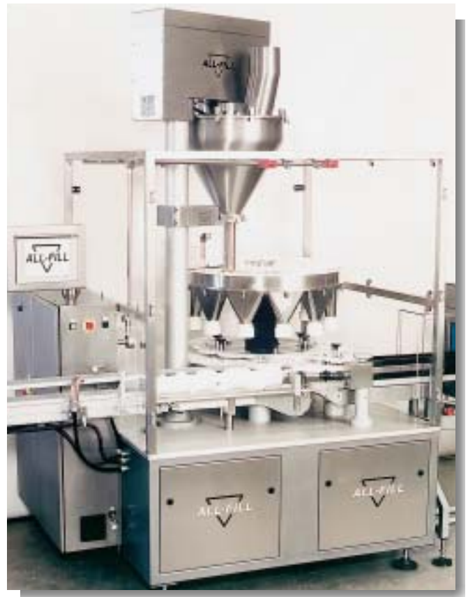
Twelve pocket continuous motion rotary filler for filling over 500 spice/herb combinations into PET catering jars at 120 jars per minute. Features the AFI 'fully sealed' filling system, adjustable vibration settling, check weigher feed-back and touch-screen control.
