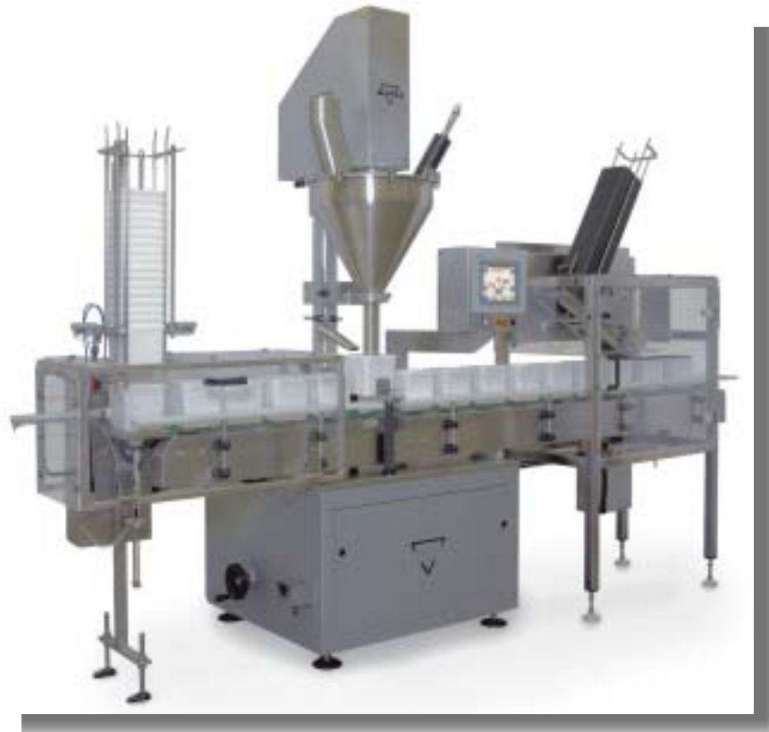
Series 100 system for bottom-up filling of food powders and bouillon paste into square and round tubs, with tub de-nesting/presentation, lifting/lowering during filling, lid de-nesting/presentation and pressing.
